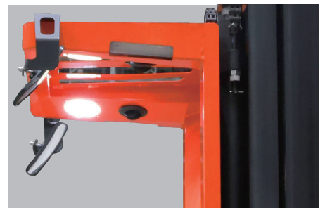
LED work lights and fan
