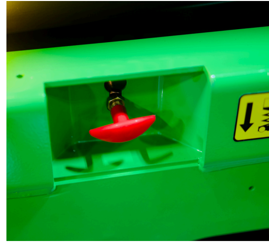
Emergency Descent System. Brings the platform down safely in the event of a power failure.
