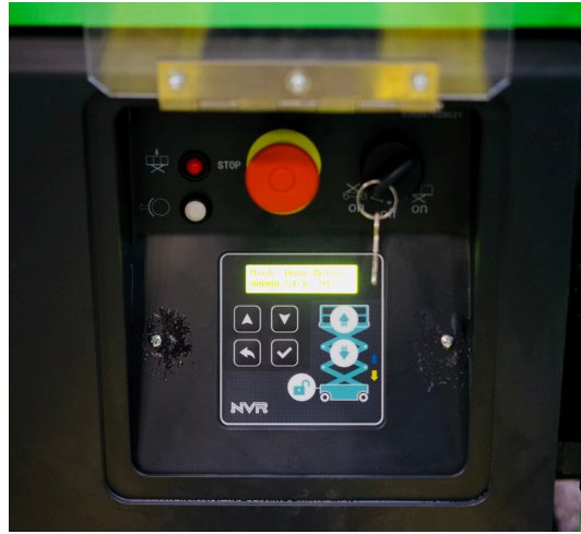
Master Power Disconnect Switch. Prevents battery drain during storage by cutting off power completely.
