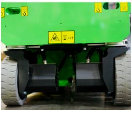
Dual Front-Wheel Drive & Steering. Enables tight turning radius and excellent maneuverability in confined areas.
