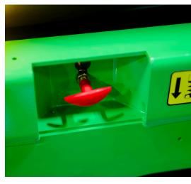
Emergency Descent System. Brings the platform down safely in the event of a power failure.
