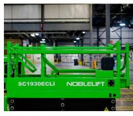
Foldable Guardrails. Allow the lift to navigate through low-clearance doorways and tight spaces.
