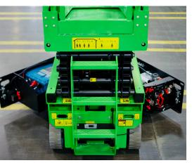
Swing-out component trays allow for easy access and maintenance.
