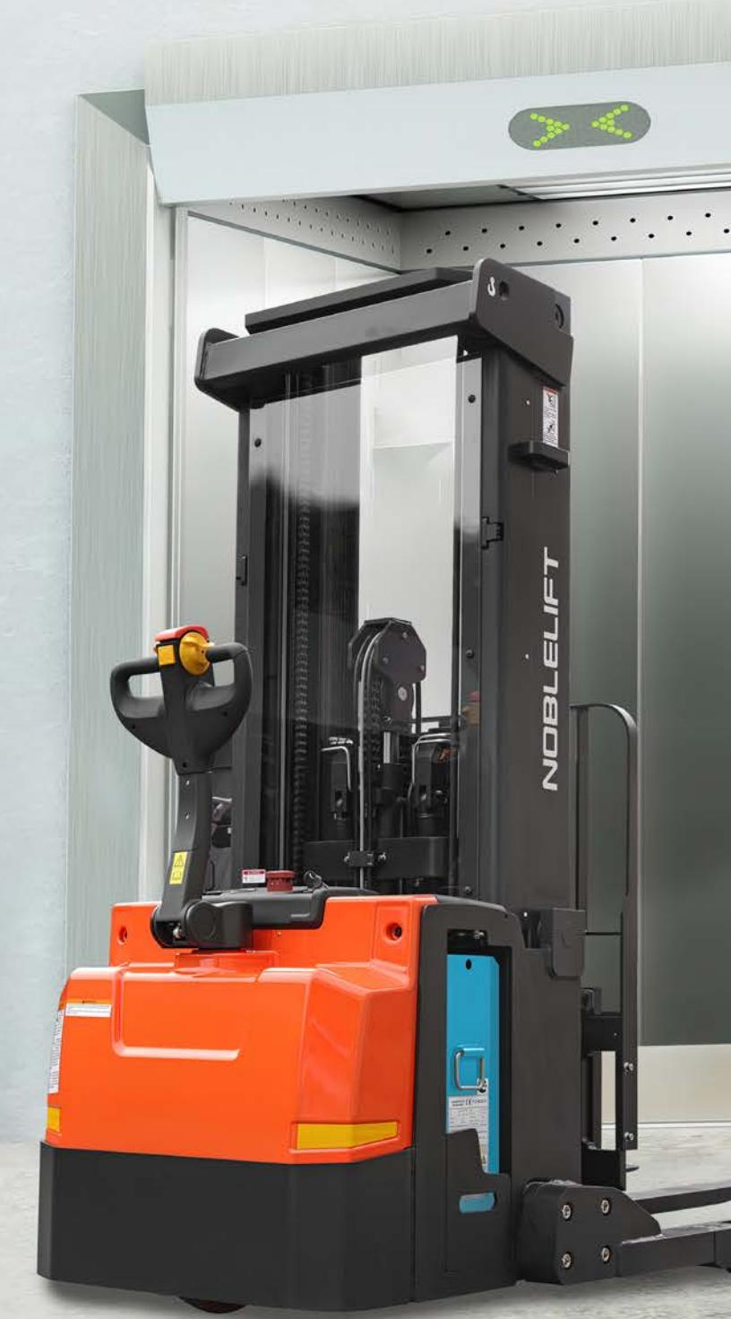
**Two-Stage Mast** - Provides 6 inches of free lift, allowing pallets to be raised off the ground without extending the mast, keeping overall height under 84 inches.
