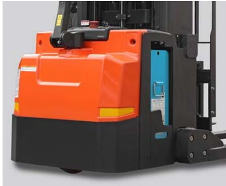
Frame is surrounded by steel to protect the truck's components and the operator's feet during work.
