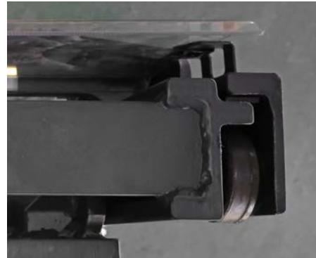
Innovative steel CJ channel mast design delivers added strength, stability and performance.
