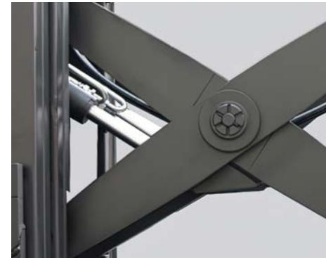
Double hydraulic cylinders provide balanced load movement and prolonged component life.
