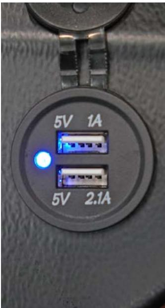
Emergency stop button. USB connector for charging and powering of additional devices during operations.
