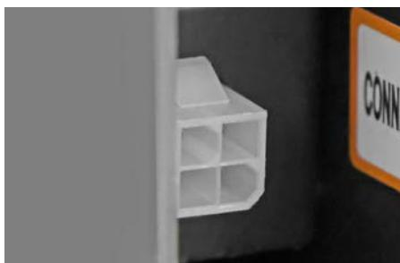
External programming port for diagnosing faults without removing the cover.
