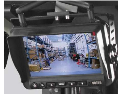
Optional fork mounted camera with HDMI color monitor provides an unrestricted view of the pallet and racking.
