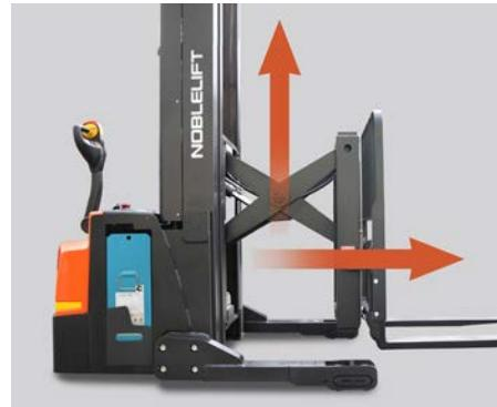
Proportional hydraulics ensure precise load positioning, while reducing the risk of product or rack damage.
