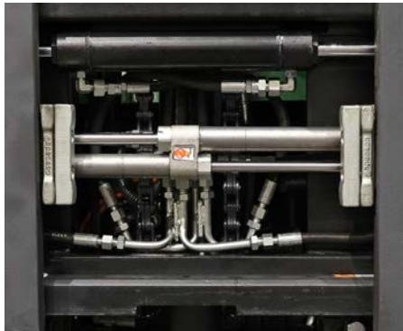
Integrated side shift allows for movement of the fork carriage without having to move the entire stacker.
