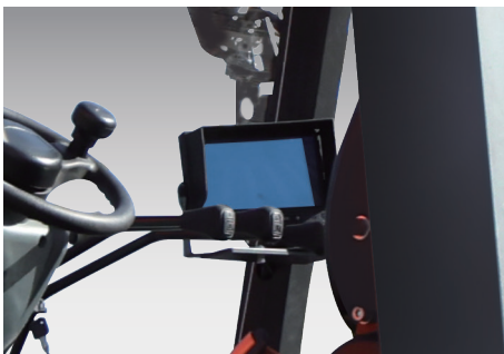
The forklift comes standard with a rearview camera, enhancing overall safety performance.
