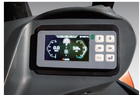
Standard color screen display shows key information such as forklift speed, working hours, battery charge, fault codes etc.
