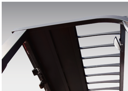
The overhead guard with integrated top cover design increases strength, ensuring safety.
