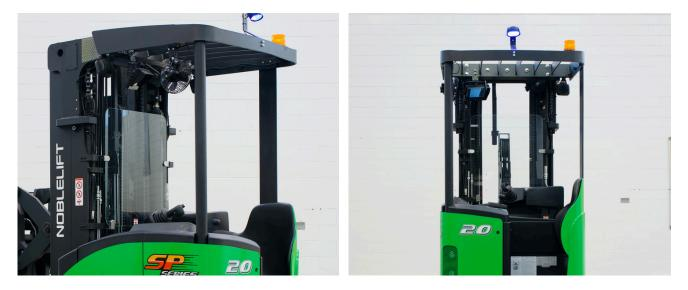
The cab design, open-view mast, and overhead guard provide the operator with a clear line of sight to the load and surroundings, enhancing efficiency and safety.
