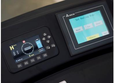
The large LED screen provides easy access to vital information, displaying lifting weight, height, speed, power, steering, fault codes, alarms, and more.
