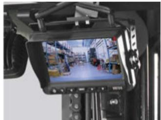
The wireless mast-mounted fork view camera with HDMI color monitor offers an unobstructed view of the pallet and racking, boosting productivity and enhancing safety.
