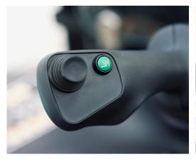
A single-button tilt control system enhances safety by restricting cargo tilt when the forks are raised.
