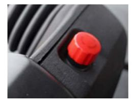
The emergency power button instantly disconnects power in critical situations, ensuring the safety of both the operator and the cargo.
