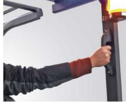
Rear grab bar with horn provides easy horn operation while traveling in reverse and keeps the operator's hand safely within the truck at all times.
