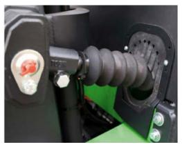
Tilt cylinder boots shield the tilt cylinder and oil seals from environmental exposure, extending the lifespan of the cylinder.
