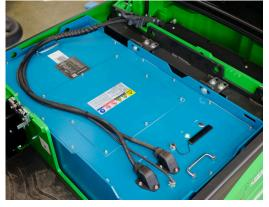
The advanced 4G wireless battery monitoring system enables remote tracking of battery performance and system data.
