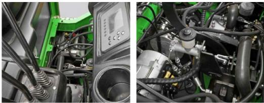
The removable floorboard offers easy access to the dual gearboxes, twin motors, and other essential components for convenient servicing and maintenance. Additionally, a detachable panel behind the seat allows access to the controllers on the lithium battery and the BMS-integrated SIM card.
