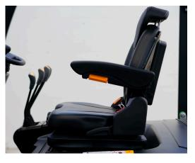
Operator Presence System (OPS) — When operator is not in seat, the hydraulic lift and tilt controls automatically lock out and traveling is disabled.
