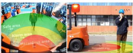
The backup camera and monitor, combined with the AI pedestrian detection system, alert the operator when a pedestrian is detected. If a pedestrian approaches too closely, the system automatically stops the forklift.
