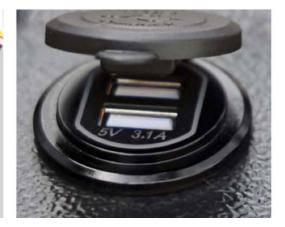
USB connector for charging and powering of additional devices during operations.
