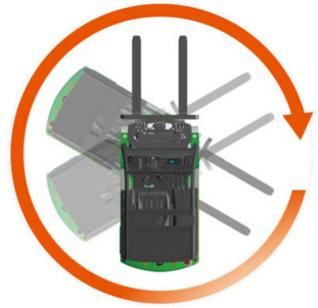
The compact design allows for a 360 degree zero-turning radius, enabling the truck to operate in confined spaces.
