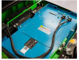
The high-capacity battery, designed for multiple shift operations, is securely enclosed within a durable steel casing.
