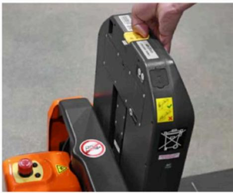
The intelligent design enables quick and effortless one-handed battery exchange in seconds.
