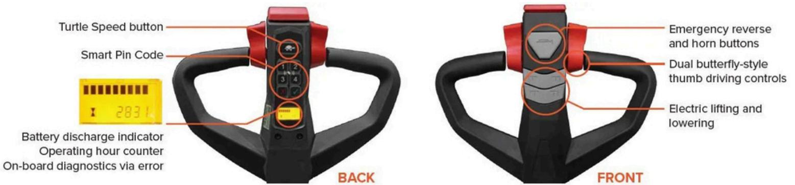
Pressing the Turtle button allows the truck to operate with the handle in an upright position (pinwheel capability), ensuring safe and efficient maneuvering in tight spaces like elevators, trailers, and containers.
