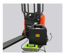
The battery supports external recharging with an optional external charger. An optional backrest is available in 42", 48", and 60" sizes.
