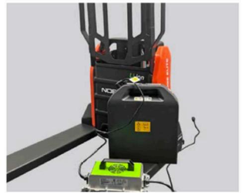
The battery supports external recharging with an optional external charger. An optional backrest is available in 42", 48", and 60" sizes.
