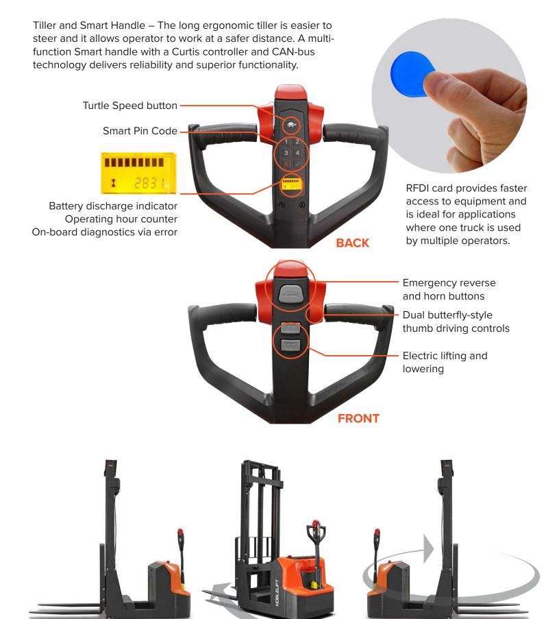
Travel speed: 2.9mph unloaded, 2.8 loaded Automatic deceleration while turning, improves safety and stability while preventing product damage.
