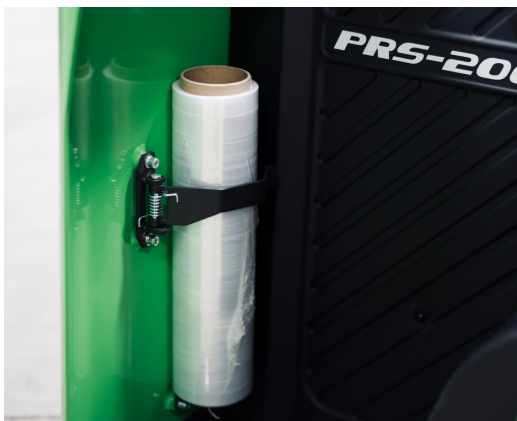
Integrated shrink wrap holder conveniently mounted onboard to improve efficiency during pallet preparation and transport
