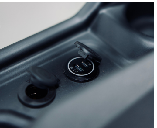
The USB & USB-C charging socket allows to power and charge mobile devices during the work.
