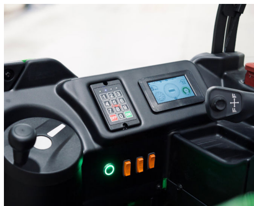
Secure operator access through key fob or PIN code, with a digital display showing steering position and truck status
