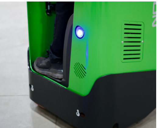
The blue spot light allows to indicate for people around the approaching truck which is increasing the safety.
