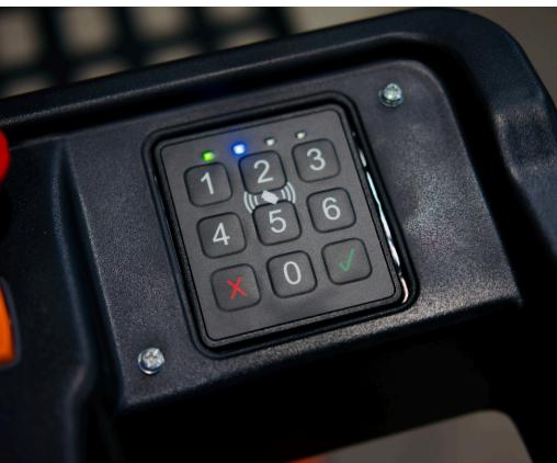
Keyless PIN code lock or RFID card access simplifies access when several users operate one truck.
