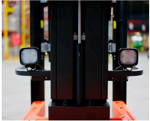
Side lights and headlight provide excellent visibility to operator even in poor lighting conditions. Vehicle is also equipped with a buzzer, warning light, rear light and safety blue light.
