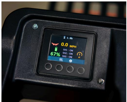
LCD display shows safety warnings, speed, steering angle and fault codes for easy operation and troubleshooting.
