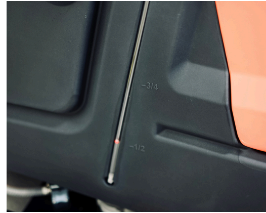
External water level indicator that shows how much clean solution remains in the tank.
