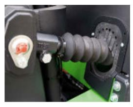
Tilt cylinder boots protect tilt cylinder and oil seals from the environment, prolonging cylinder life.
