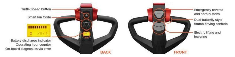
Pressing the Turtle button allows the truck to operate with the handle in an upright position (pinwheel capability), ensuring safe and efficient maneuvering in tight spaces like elevators, trailers, and containers.
