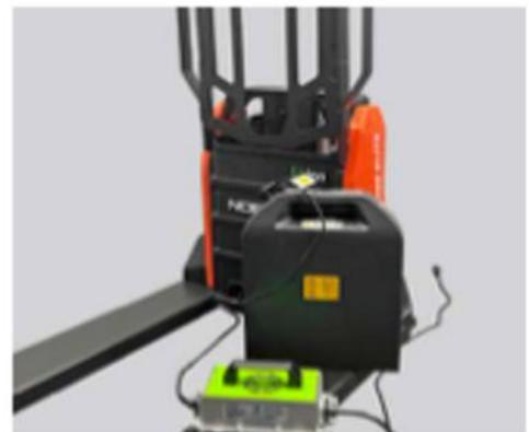
The battery supports external recharging with an optional external charger. An optional backrest is available in 42", 48", and 60" sizes.
