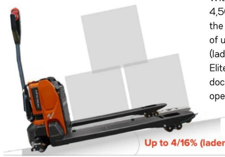
With a capacity of up to 4,500 lbs (2000kg) and the ability to tackle ramps of up to 4/16% (laden/unladen), the EDGE Elite is perfect for loading docks and delivery operations.
