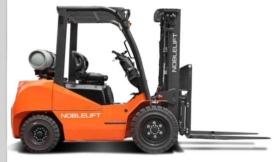
Modular frame is designed based on the same chassis as the NOBLELIFT Diesel and Electric forklifts. Main components and configurations are the same. Spare parts inventory is minimized to reduce service and maintenance costs.
