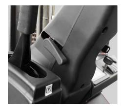
The angle of the steering column is easily adjusted with a lever on the left-hand side of the steering column.
