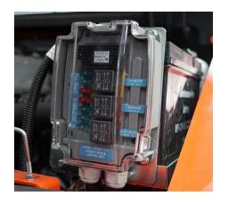
Durable controller that integrates all electrical components is protected from temperature, water and vibration.
