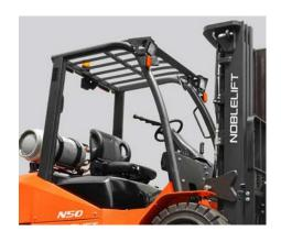
Heavy-duty steel chassis, axles, mast and overhead guard deliver high strength and stability for high lifting heights and heavy loads.
