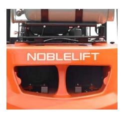
Angled exit ports direct engine air away from the operator and the cab to help operators stay cool.
