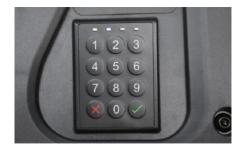
The Pin-Code lock can be set with multiple passwords and also supports RFID card activation.
