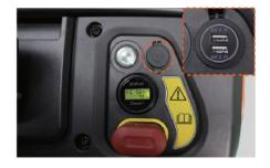
The multifunctional-LCD indicator displays the information about remaining battery power, amount of working hours and fault codes. Built in USB port for charging other devices
