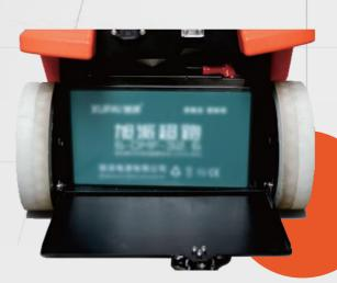
Low energy controll system, one full charge can keep machine running 1.5~2 hrs with standard 24V32AH lead-acid battery.
