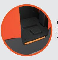
The floor suspension system adapts to the weight of operator and provides impact and vibration protection.
