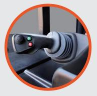
The multifunctional integrated handle not only has lifting, lowering, tilting and side shifting, but also forward and backward shifting through the handle control, which is fast and convenient to use.
