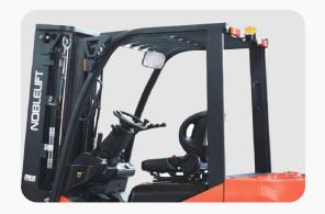
The rear assist grip with a horn enhances comfort by offering easy horn operation while trevelling in reserve.
