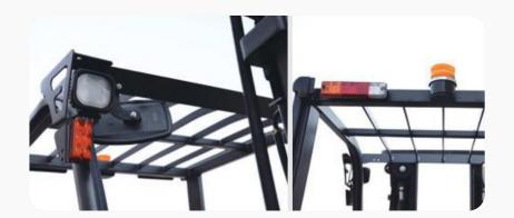
The forklift is equipped with standard LED lamps
