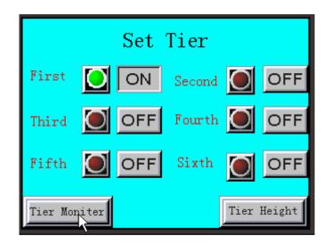
Click "**Tier Moniter**" button to enter the Tier Monitor page, then operate the lifting handle, the forks start to lift until reach the selected tier and delay for a period of time (the time length can be set in the "parameter setting". If the lifting handle is not released after the delay, the truck will automatically switches to manual function and continues to lift).
