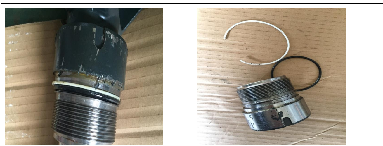
4. Remove o-seal and shield ring, then repair hose . Installation way is in reverse sequence
