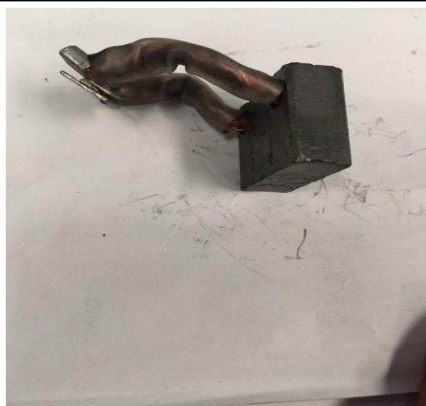
3. Unscrew the screw with a cross screwdriver and take out the carbon brush and replace it. Installation process and the inverse process of the above process.
