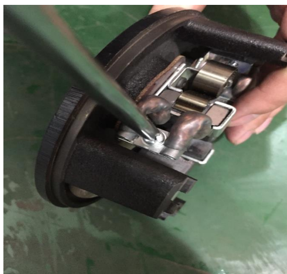
3. Unscrew the screw with a cross screwdriver and take out the carbon brush and replace it. Installation process and the inverse process of the above process.
