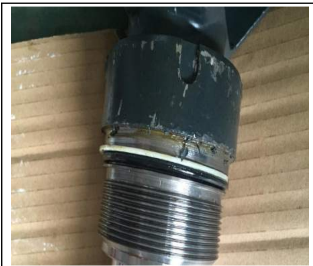
3. Remove o-seal and shield ring, then repair hose. Installation way is in reverse sequence
