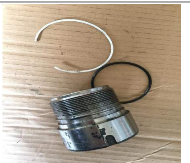
3. Remove o-seal and shield ring, then repair hose. Installation way is in reverse sequence
