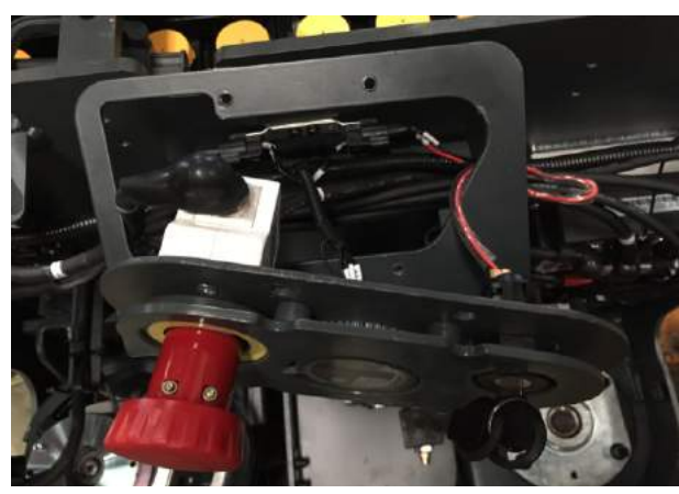
11. Remove the instrument panel by unscrewing the four screws with a 6mm inner hexagon wrench.
