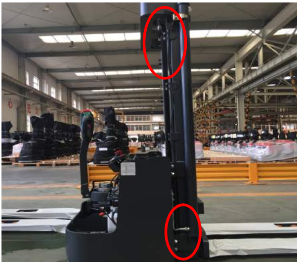
1. Remove the oil pipes at the lifting cylinder on both sides with 19mm open spanner. Note: hydraulic oil will leak out when removing the oil pipes.
