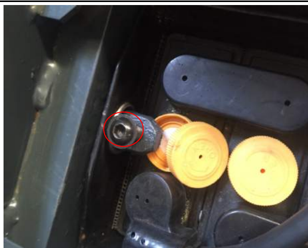
3. Unscrew the bolt with the 5mm inner hexagon wrench
