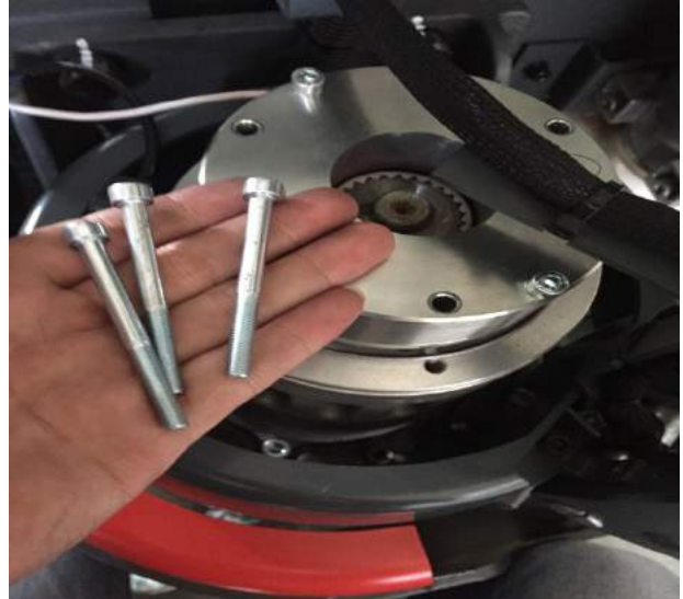
2. Unscrew the 3 bolts of installing the brake with 4mm inner hexagon wrench
