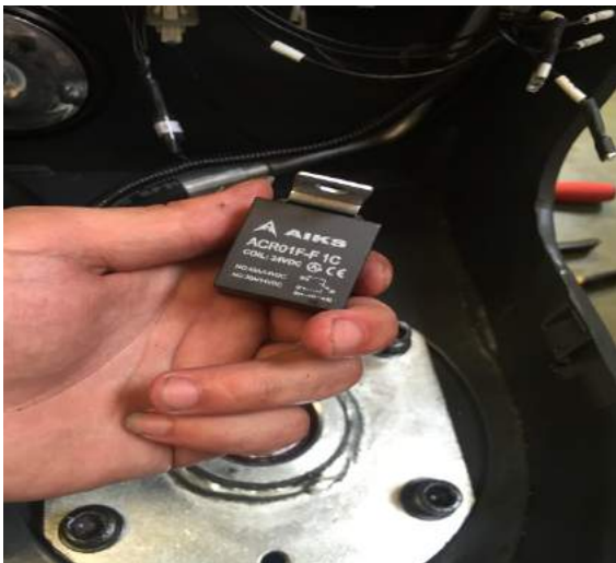
3. Relays can be replaced, and the installation process is the reverse process of disassembly
