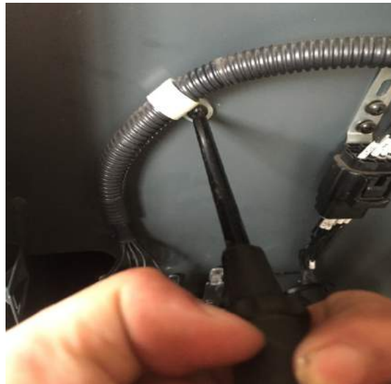
14. Unscrew the wire harness holder with a 14mm cross screwdriver
