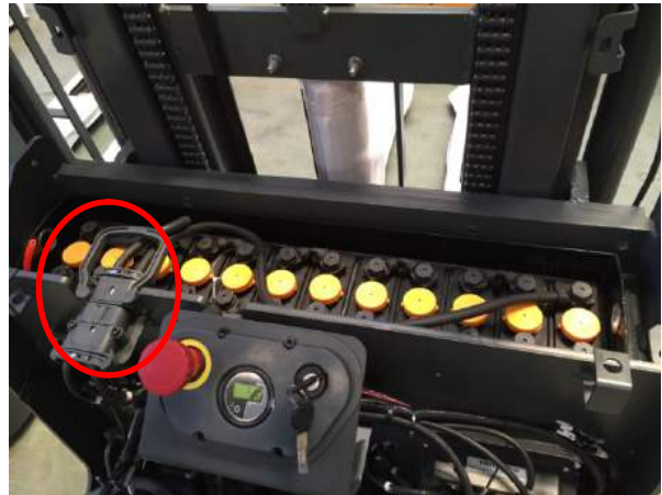
2. Disconnect the power supply of the vehicle, i.e. unplug the battery connection port in the picture below.
