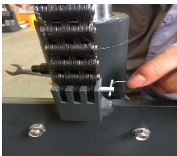
2. Remove the cotter pin from the top of the chain
