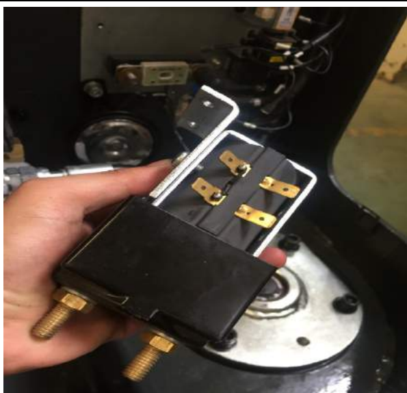
7. Remove the contactor with mounting frame
