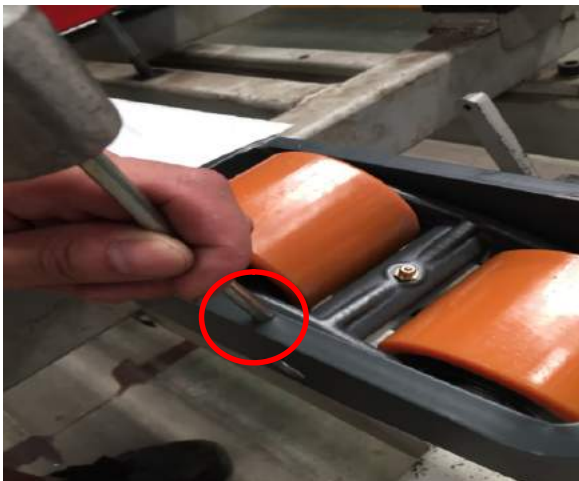
3. Place the body on the repair rack and remove the elastic cylindrical pin with a punch.
