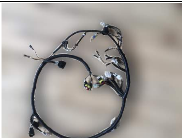
13. Unplug each plug in turn. This plug is one-to-one corresponding
