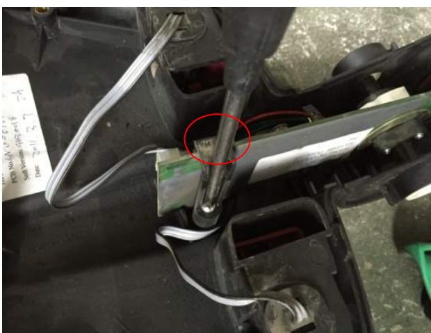
3. Unscrew the screw fixing the drive switch with a 2mm inner hexagon wrench
