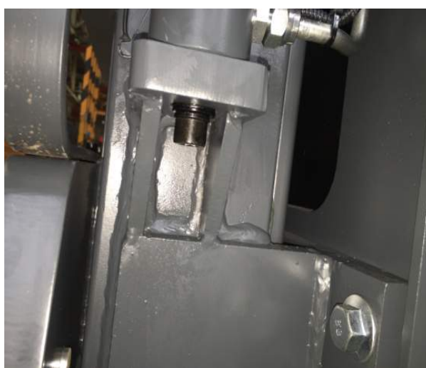
5. Remove the fixing bolt of the cylinder base with a 12mm inner hexagon wrench.
