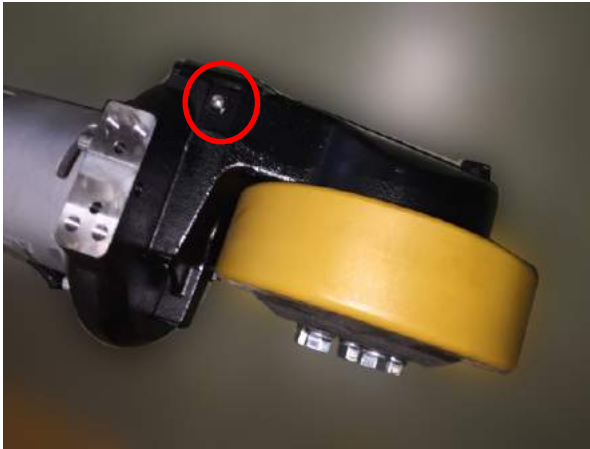
1. There is an oil injection hole on the front of the driving wheel
