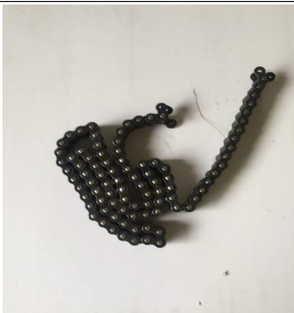
5. Remove the chain and replace it. The installation process is the reverse process of disassembly
