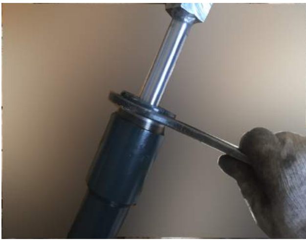
1. Unscrew the oil cylinder head with a crescent wrench.
