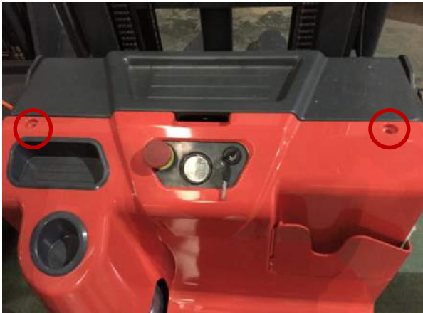
1. Remove the bolts shown below with an inner 6mm hexagon wrench.
