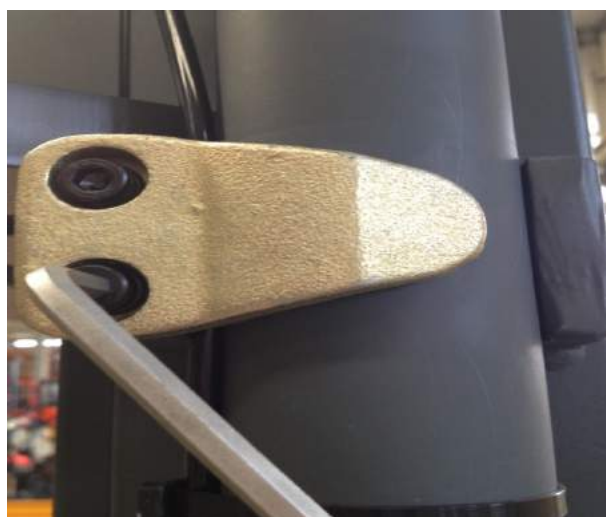
4. Using the 6mm inner hexagon screw down the cylinder pressure plate fixing bolt
