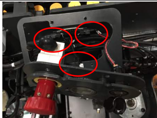
2. Disconnect the power supply of the vehicle, i.e. unplug the battery connection port in the picture below.
