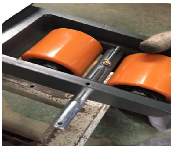
4. Remove the axle and remove the entire component.
