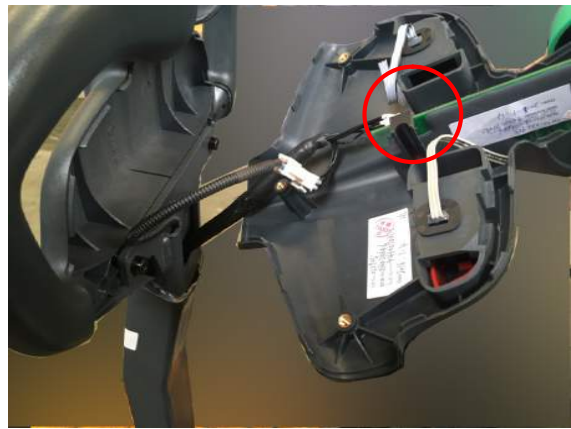
2. After unscrewing the screw, carefully open the handle housing and unplug the connecting plug
