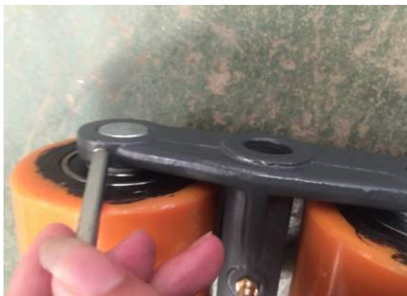
5. Take out the elastic pin with punch
