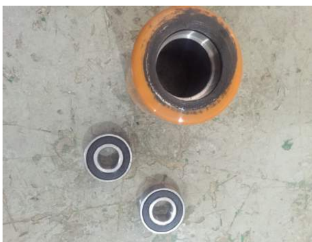
7. Take out the two bearings with the punch and then repair and replace them. The installation process is the reverse process of disassembly.
