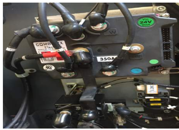
10. Unplug all plugs on the right side, which are one-to-one corresponding.
