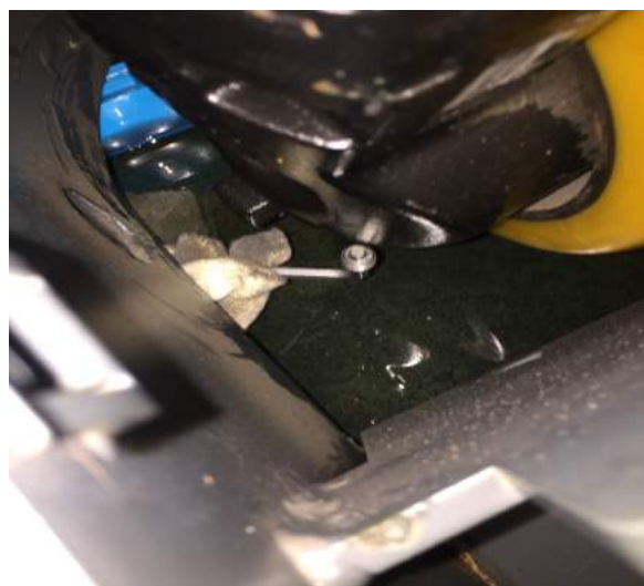
4. Unscrew the bolt of the oil drain hole at the bottom with the 7mm inner hexagon wrench, and quickly place the waste oil collection container at the bottom to collect the waste oil, so as to avoid the waste oil flowing out and polluting the environment. When the waste oil runs out, screw on the bolts.
