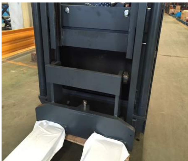
7. Raise the maste and remove the tray frame.
