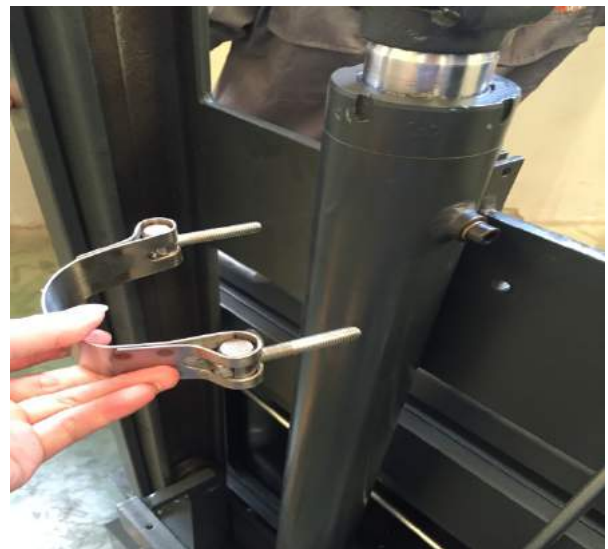
5. Unscrew the hoop bolt with a 13mm open wrench and take the hoop
