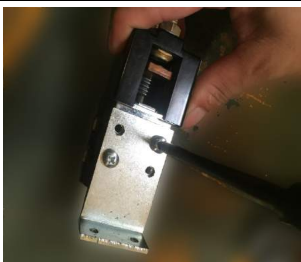
8. Unscrew two screws with a screwdriver.
