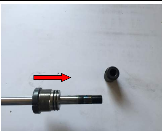
3. Remove the piston with pipe tongs. Heat the connection between the piston and the piston rod before using the pipe tongs because there is threaded glue inside.
