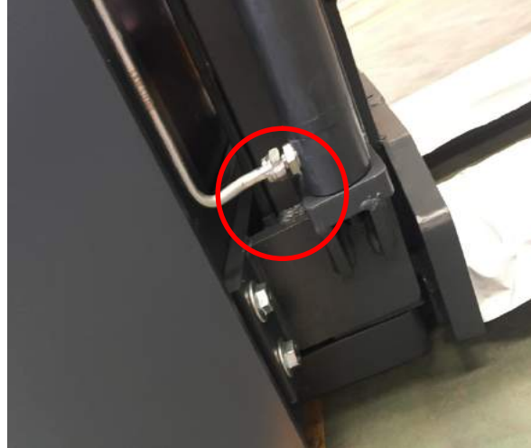
1. Remove the oil pipes at the lifting cylinder on both sides with 19mm open spanner. Note: hydraulic oil will leak out when removing the oil pipes.
