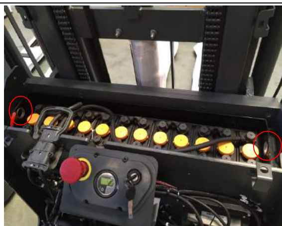
3. Use a tool to connect here, such as a hook, and then remove the battery
