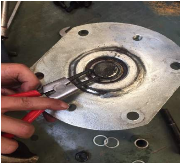
1. Remove the clamp spring with clamp pliers
