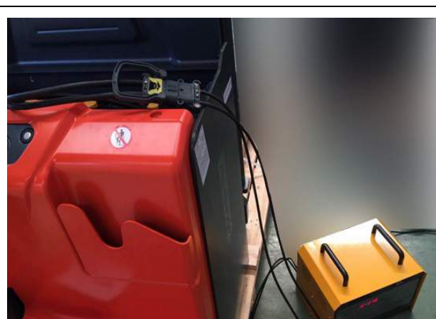
1. The connector of the product is connected with the connector of the charger to charge the battery.
