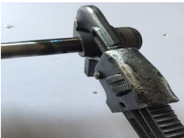
3. Remove the piston with pipe tongs. Heat the connection between the piston and the piston rod before using the pipe tongs because there is threaded glue inside.
