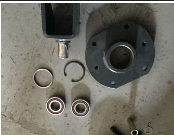
5. Take out the axle, sleeve, clamp spring and other parts, can be replaced and maintained, the installation process is the reverse process of disassembly.
