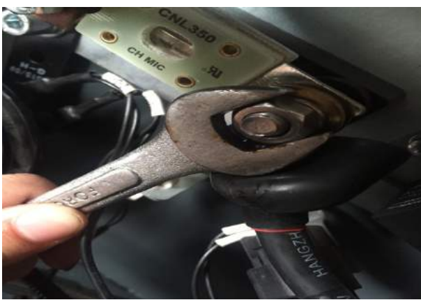
3. Unscrew the screw with 13mm wrench, unplug the plug, and write down the line number
