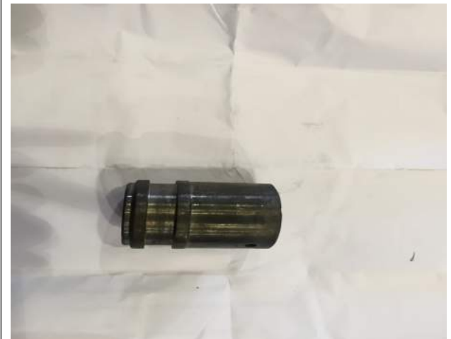
3. Remove the piston with pipe tongs. Heat the connection between the piston and the piston rod before using the pipe tongs because there is threaded glue inside.
