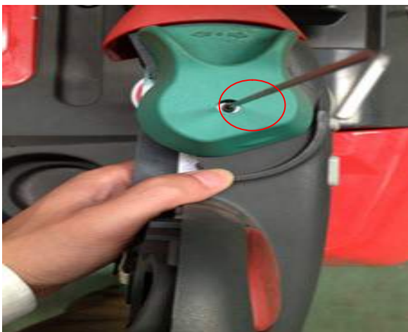
3. Unscrew the screw fixing the drive switch with a 2mm inner hexagon wrench
