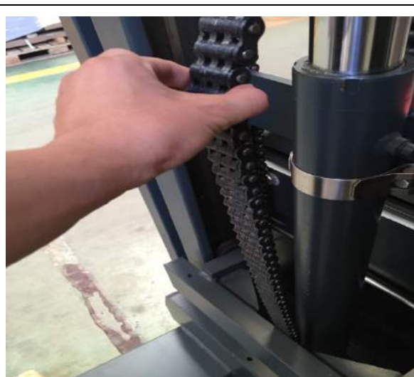
1. Lift the tray rack and pad it with wood, so that the chain can reach the state of no stress
