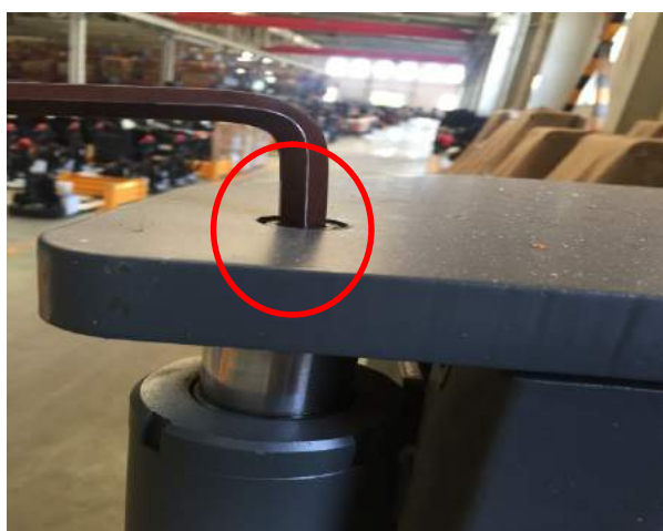
3. Remove the bolt at the top of the oil cylinder by the 12mm inner hexagon
