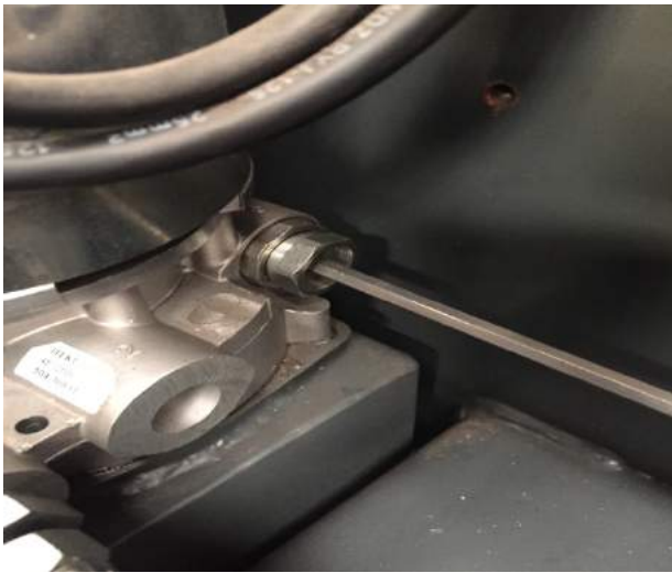
3. Adjust the pressure of the oil pump with a 6 mm inner hexagon wrench
