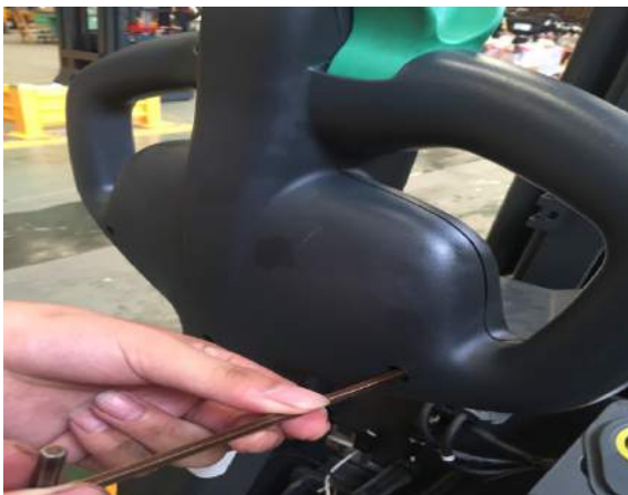
1. Unscrew the outer cover screw with 6mm inner hexagon wrench
