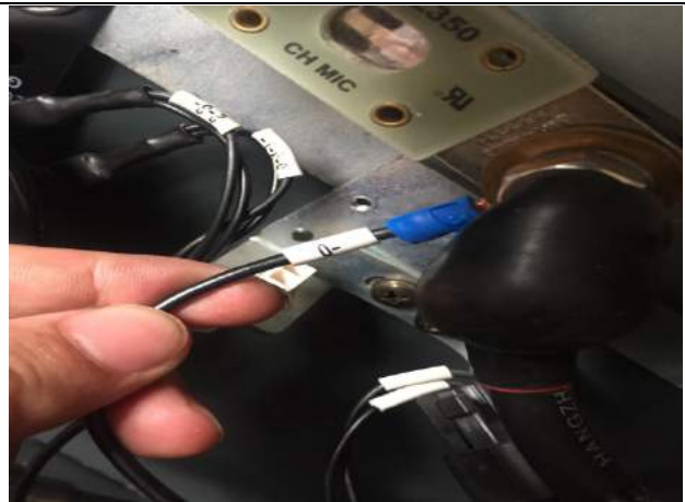
3. Unscrew the screw with 13mm wrench, unplug the plug, and write down the line number
