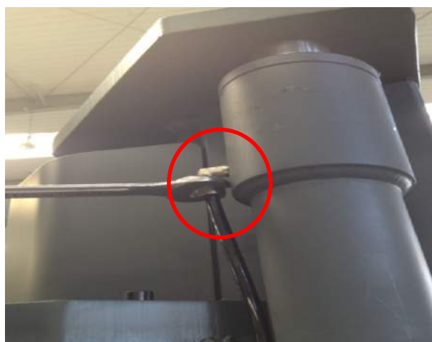
2. Use a 12mm wrench to remove both sides of the return tubing
