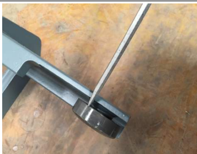
4. Use the punch to remove the roller so that it can be replaced
