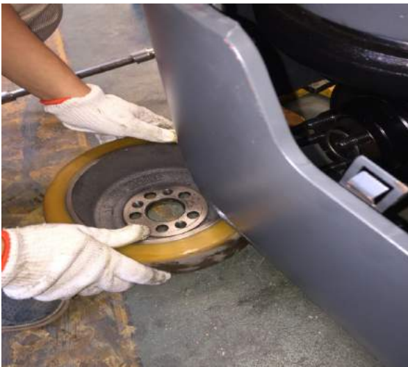
5. Take out the driving wheel from the bottom and replace it. The installation process is the reverse process of disassembly.
