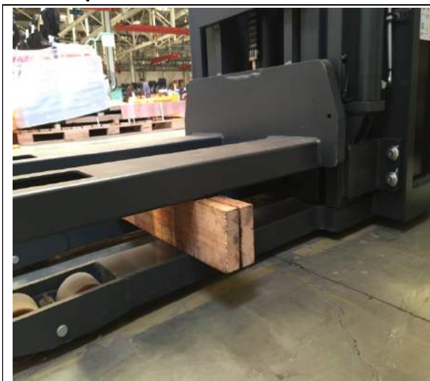
1. Lift the tray rack and pad it with wood, so that the chain can reach the state of no stress
