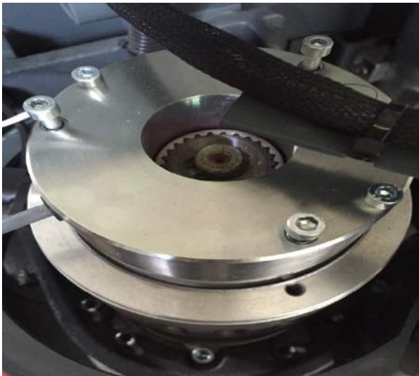
2. Unscrew the 3 bolts of installing the brake with 4mm inner hexagon wrench
