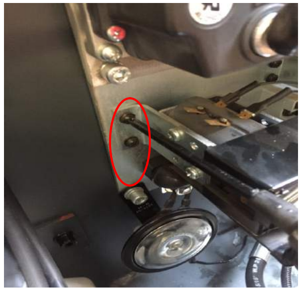
6. Unscrew the two screws with a cross screwdriver
