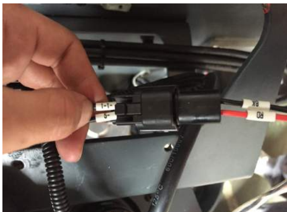
12. Unplug the plug one by one and write down the line number
