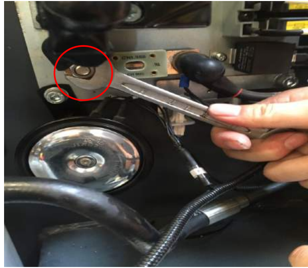
4. Unscrew the bolt with a 13mm open end wrench
