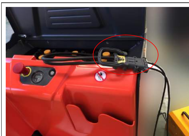
1. The connector of the product is connected with the connector of the charger to charge the battery.
