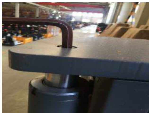
3. Unscrew the fixing bolt at the top of the oil cylinder with a 12mm inner hexagon wrench
