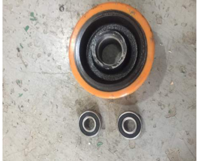
3. When the axle is removed, the axle and other components of the wheel group can be replaced. The installation process is the reverse process of disassembly
