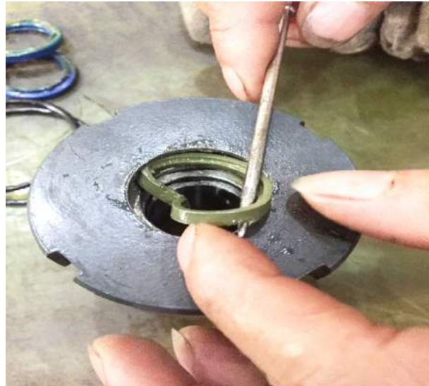
5. Take out the Stepseal, the oil cylinder head sealing ring can be disassembled and replaced
