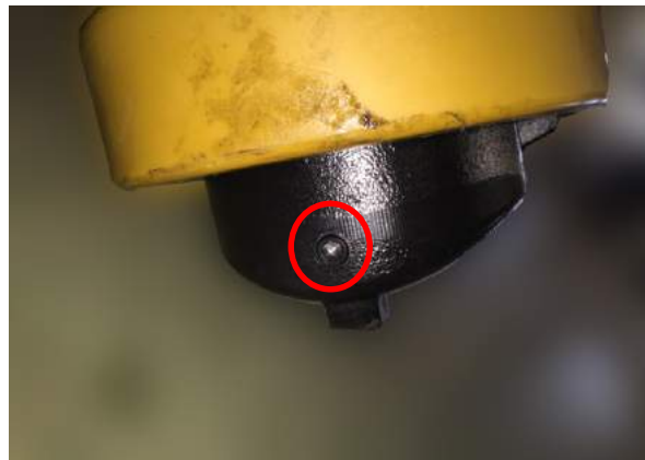
2. There is an oil drain hole at the bottom of the driving wheel.
