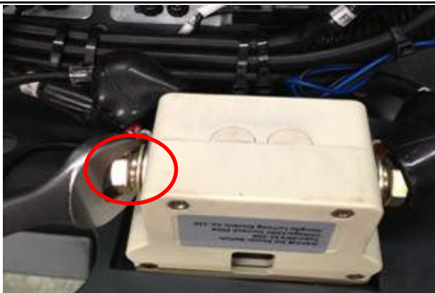
3. Unscrew the four screws with the 6mm inner hexagon wrench, and cut off the binding belt of the surrounding wiring harness
