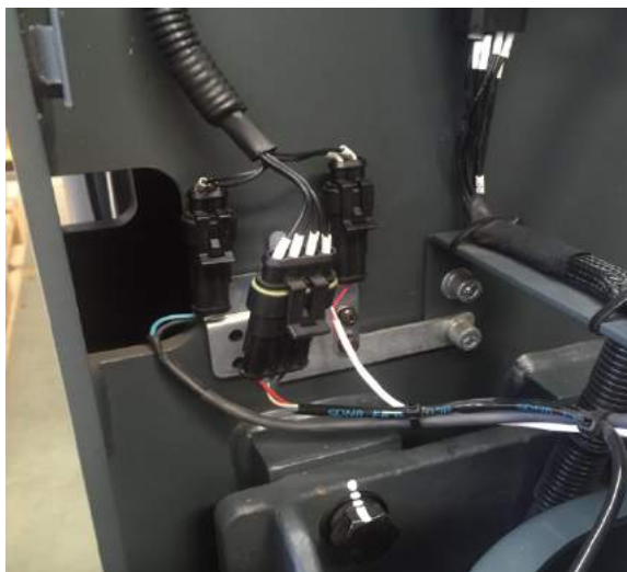
3. Take out the connecting plug from the cable mounting frame.
