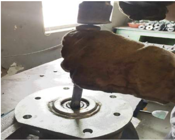
2. Remove the wheel frame with punch
