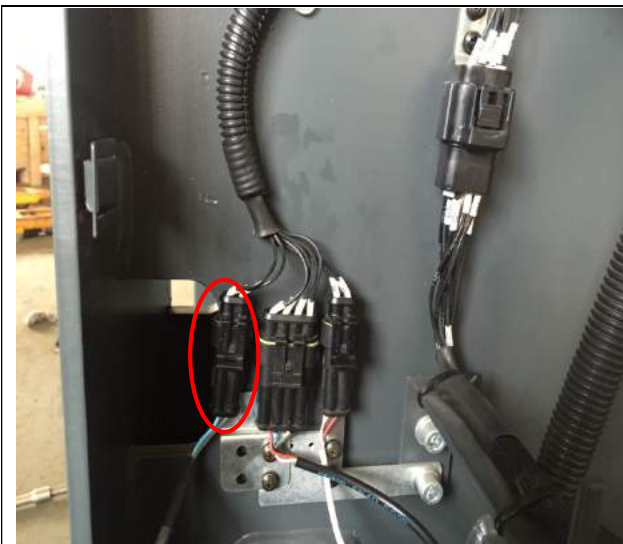
3. Unplug the plug and cut the tie
