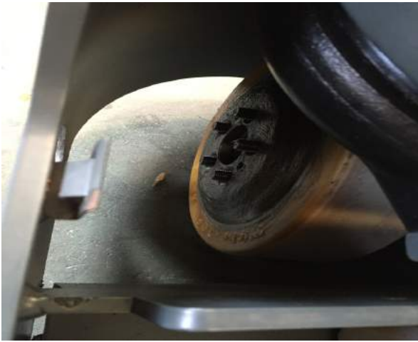
4. Remove the wheel by unscrewing five retaining bolts.
