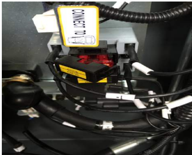
2. After opening the fuse box, take out the old fuse, replace the new fuse, the installation process and the reverse process of the above process.
