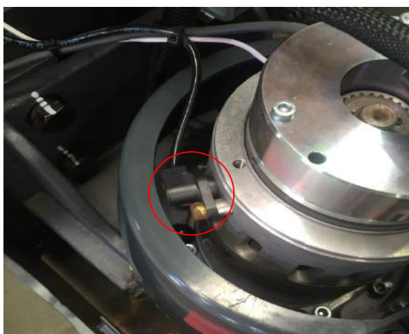
1. Unscrew the fixing bolt with 4mm inner hexagon wrench
