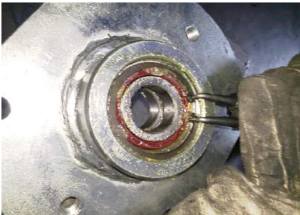
3. Take out the clamping spring at the bottom of the bearing seat with clamping spring pliers.
