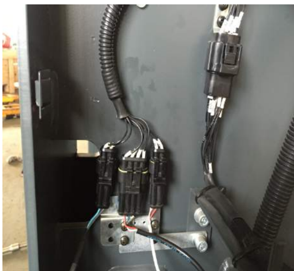
13. Unplug each plug in turn. This plug is one-to-one corresponding
