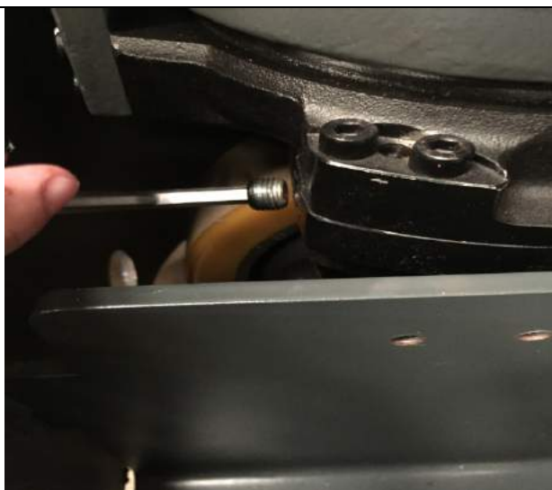
5. Use a 7 mm hexagon socket wrench to unscrew the oil hole bolts
