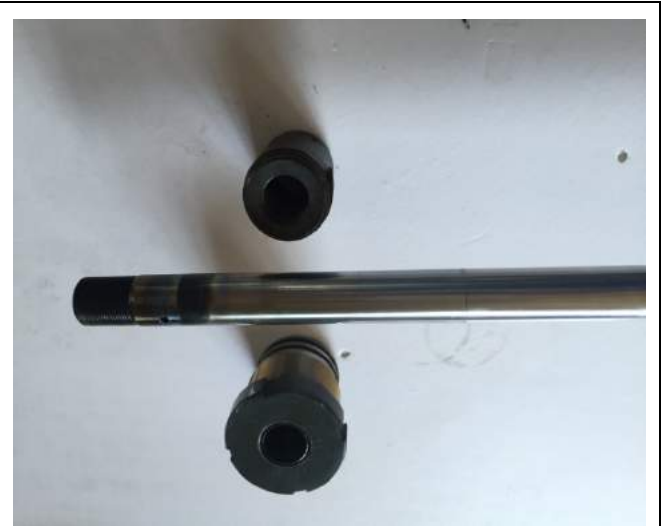
3. Remove the piston with pipe tongs. Heat the connection between the piston and the piston rod before using the pipe tongs because there is threaded glue inside.
