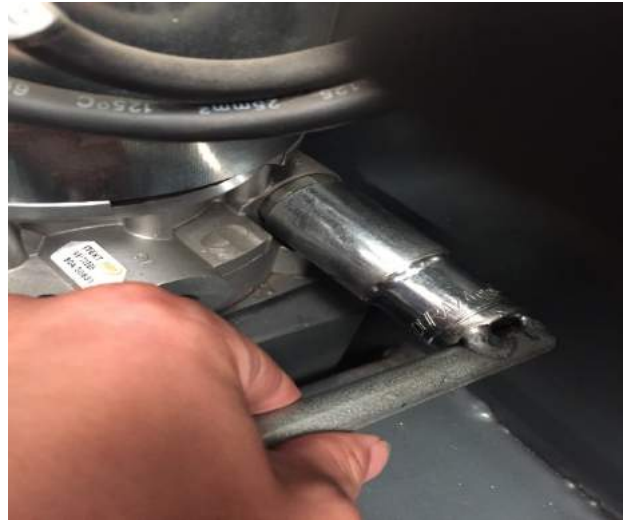
4. Tighten bolts with a 24 mm hexagon socket wrench
