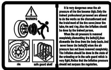
Tyre removal signs
