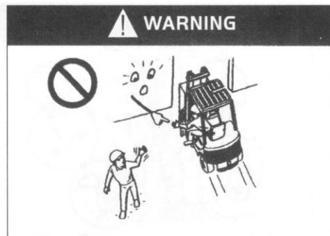
Do not put arm and body outside of the overhead guard during work!
