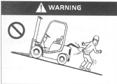
Do not park the forklift on the slope!
