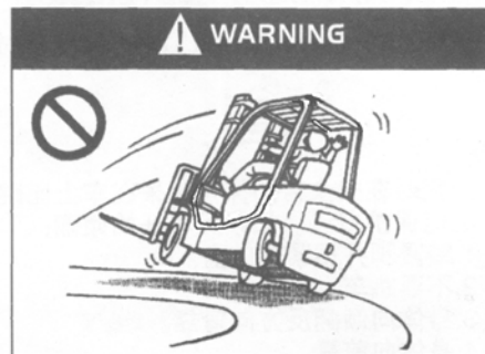
whether load or no-load, don't turn in a high speed or in a large radius!
