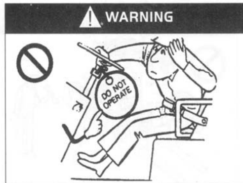
Do not drive an unsafe forklift!
