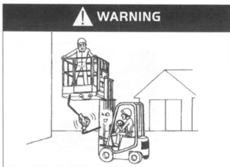
Must use special equipment to lift people safely to work at height!
