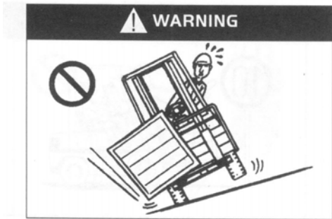
Not turn when driving on a slope!
