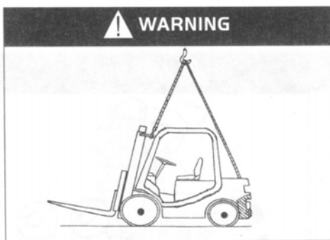
Hoisting the forklift correctly!
