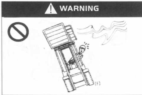
Do not lift when there is excessive wind!
