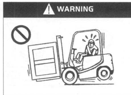
Do not overload!
