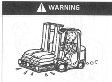
Use appropriate pallets or sleeper when handling small objects!
