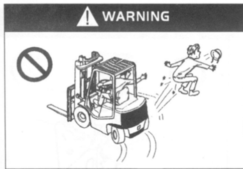
Pay Attention Not To Touch People Or Object When Steering Do Not Approach To Forklift When Its Working
