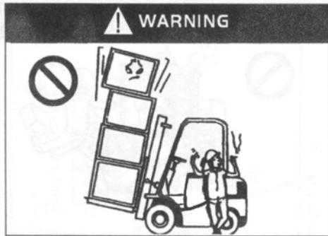
Try To Prevent Loads From Exceeding Backrest Fasten The Goods Which Is Difficult To Bind Before Loading
