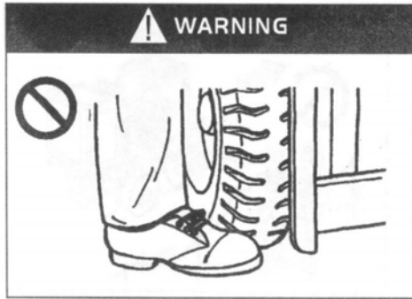
Do Not Move Forklift When There Is People In The Front No Walking Or Standing Under Lifted Fork
