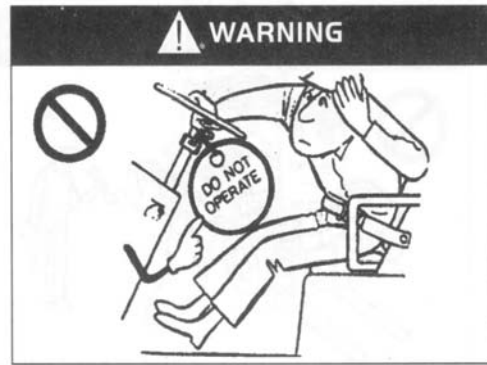
Do Not Drive Unsafe Forklift
