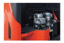
The low noise gear pump can reduce the lifting noise. The truck adopts the brand moving motor controller, oil pump motor controller and steering motor controller, so it has the characteristics of self-protection, maintenance-free, and superior performance.
