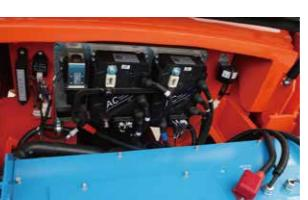
Controller assembly located on higher position for easy ventilation and maintenance.
