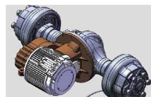
Drive system uses a horizontal fan-shaped drive axle arranged in parallel with a large transmission ratio. The battery is located at the bottom of chassis, the truck has good stability. Drive motor uses AC maintenance-free motor. Long wheelbase(1700mm)design, better stability.
