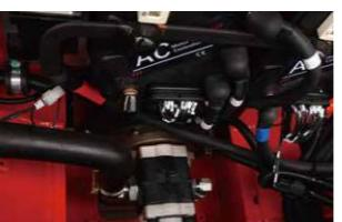
Lifting Motor located in high position so the truck can work in applications where there are water on the ground.
