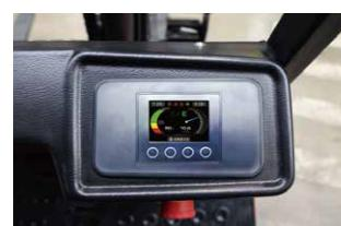
Ergonomically designed LED display with large screen and great visibility for easy control and operation with all around truck status information.
