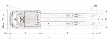
1). After the fork descent x=1600mm, y=2788mm; 2). Install crash pads 11=3810mm, 12=1409;
