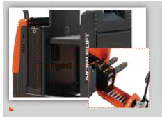
Sideways battery exchange compartment plus adjustable handling bracket makes battery replacement easier and quicker.
