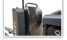
the backrest ensure the operator not to be thrown off while the stretch film, art knife, marker pen, or other truck turns at high speed. This design greatly improves the tools. safety of driving. Meanwhile, the handle above the backrest provides a grasping point for the operator when get up or down the truck, provides superior comfort for the operator.
