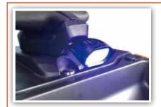
The standard blue light does not only automatically lit while the ruck forwarding but also follows the handle to turn while the truck turns. It greatly improves the safety of the operation.
